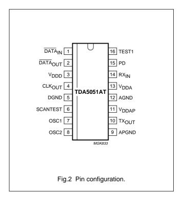
All logic inputs and outputs are compatible with TTL/CMOS levels, providing an easy connection to a standard microcontroller I/O port.
